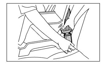
3. Buckle the belt. Make sure the release button is positioned so you would be able to unbuckle the safety belt quickly if you ever had to.
